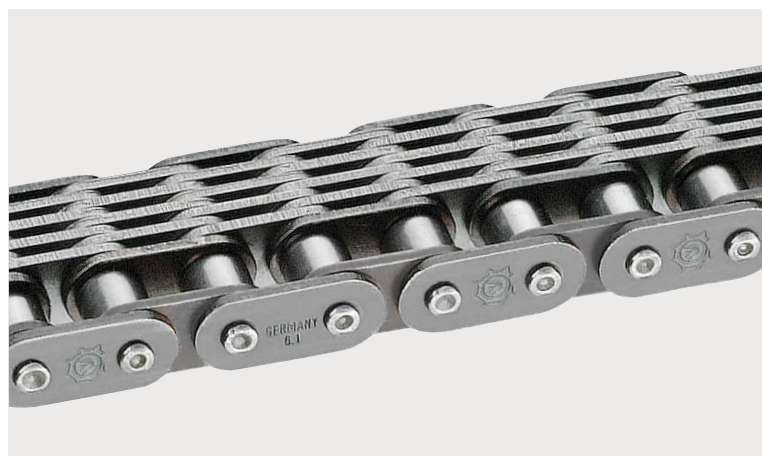
Special chain as combination of leaf chain (support) and roller chain (drive) Application: Materials handling
