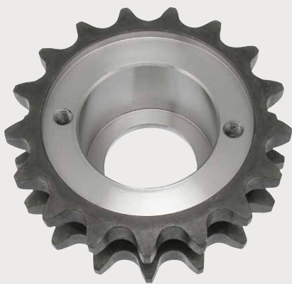
Sprocket with inductively hardened toothing, special hub and tapped bore
