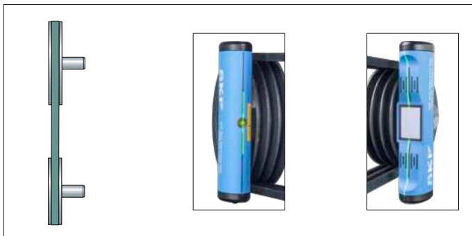
Figure 9 Pulleys perfectly aligned
